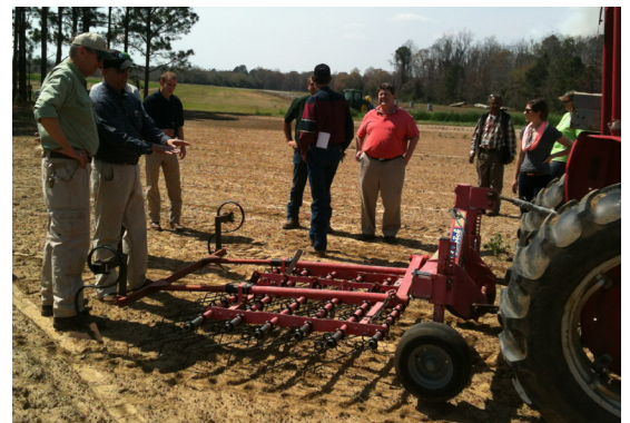
A tine weeder is used to prepare a stale seed bed before planting.
